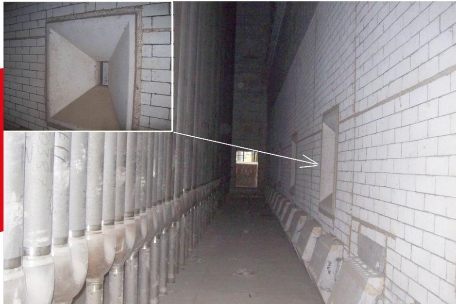
**Insulvac® vacuum formed shapes** (up to 1600°C) are manufactured by vacuum forming a mixture of ceramic, low bio-persistent or polykristaline fibres, with specially selected organic or inorganic binders.
