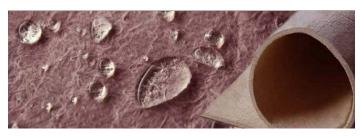
(CUI). Hydrophobic and breathable, **Pyrogel® XTE** ensures long-lasting water resistance for both the insulation layer and underlying asset; they remain drier for longer, preserving process conditions, and saving energy in the harshest of environments.
